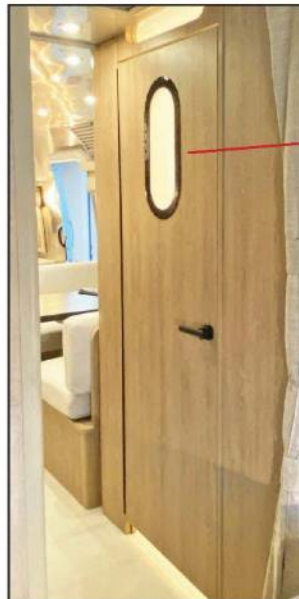
ASS'Y Bath Door with Port-hole: 969658 Utilize: 365249 TAPE ONLY FOR GLASS ASSY, NO SCREWS OR RIVETS
