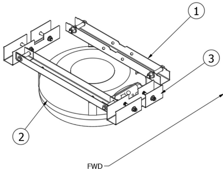
113172      Install, LP Tank, Toroidal (not for order/see parts below)
