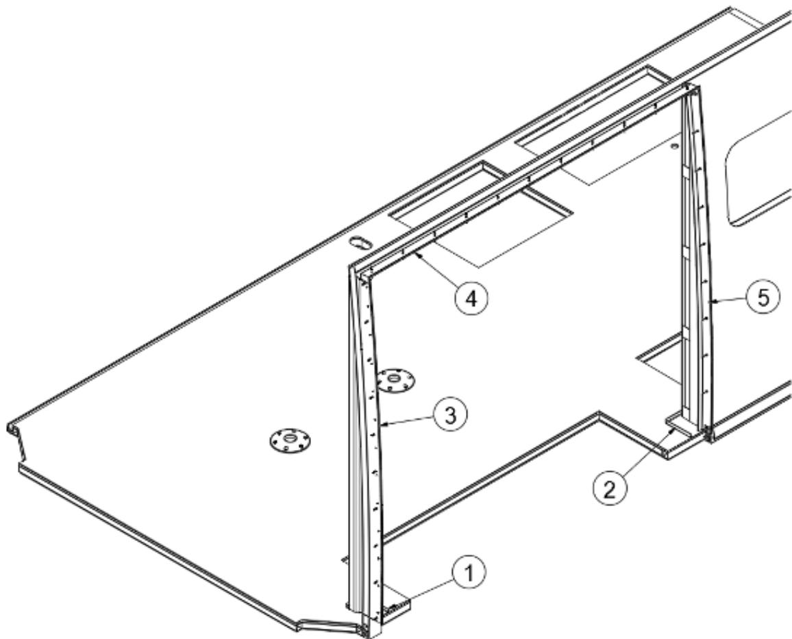
112425      Slide-out Sidewall Extrusions Install (not for order/see parts below)
