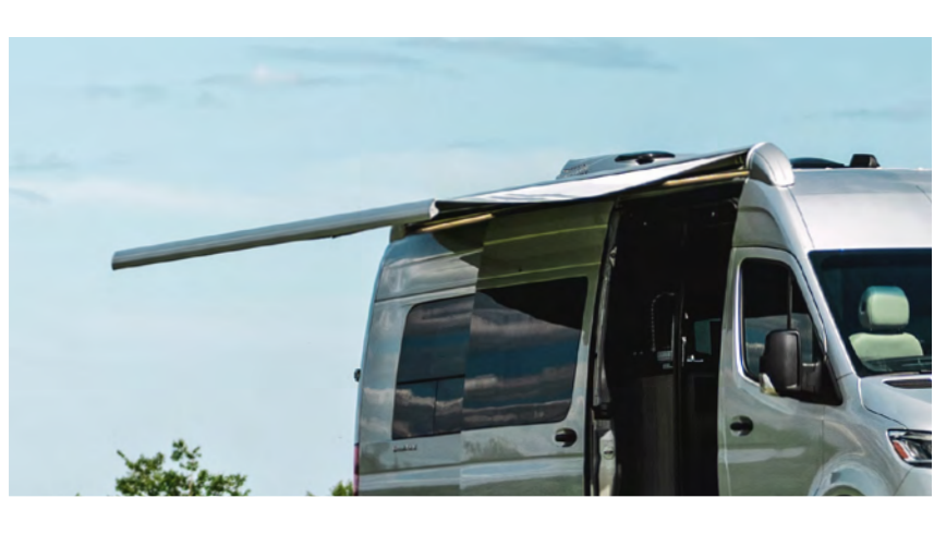
2 The powered awning extends and retracts at the push of a button.
