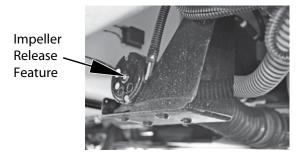
After long periods of non-use, a stuck impeller can be easily broken loose with a screwdriver inserted in the motor shaft slot. Remove the rubber boot, turn the shaft clockwise, and replace the rubber boot. The impeller can usually be found under the touring coach, near the macerator hose reel.
