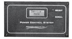
The display panel requires little user interaction and is provided to help the user understand power management. The display monitors the total AC current of the touring coach and prevents circuit breaker tripping by momentarily shedding loads. As additional appliances are turned on the system will begin to shed loads. As appliances are turned off, and a minimum of two minutes has expired, the system will automatically restore power to each of the shed loads.
