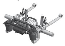
The touring coach is equipped with a rear axle air suspension. The Mercedes-Benz Sprinter Van is extremely suited for this air suspension system.
