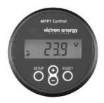
The rooftop solar panels installed on your Airstream help maintain battery health, reduce operating expenses, and extend the battery life of the batteries. The solar system's solar charge controller gathers energy from the individual solar panels and stores it in your batteries. The system features a display (shown above) that allows you to view live status information like solar watts and battery voltage.
