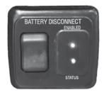
The battery disconnect switch is used to separate the batteries from the 12-volt distribution panel and converter charging system. The Atlas battery disconnect switch is equipped with LED indicators. When the light is green the switch is ON and the batteries are charged. When the red LED begins to blink slowly it is an indicator the batteries should be charged. If the red LED begins blinking rapidly the batteries should be charged immediately before battery damage incurs.
