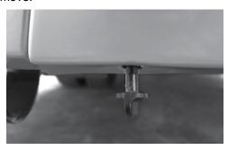
3. Pull straight down to remove the cover. Once removed you can store this in one of the utility compartments. Reverse these instructions to reinstall.
