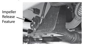
After long periods of non-use, a stuck impeller can be easily broken loose with a screwdriver inserted in the motor shaft slot. Remove the rubber boot, turn the shaft clockwise, and replace the rubber boot. The impeller can usually be found under the touring coach, near the macerator hose reel.
