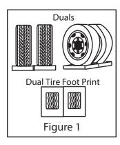
The CORRECT methods are shown in Figure 1. Dual tires are supporting the full load. Please note that the blocks are wider than the tread and longer than the tire's footprint. This provides maximum support to the tires and ensures that the load is evenly distributed throughout the tire's footprint area.
