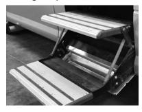
The curbside door has a folding double step with auto retract, step out warning buzzer, and a lock extended switch located just inside the door. Please read, understand, and instruct passengers of the following operational and safety information pertaining to the step.
