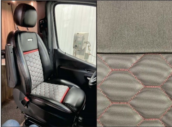
704837-D+P Front Driver + Passenger Recovers: Main body UL is 704602 Loam-Crow, combined with 704830 Simtex-Crimson red accent vinyl, and 704268 Reef-Stone hexagonal stitched insert with red contrast threading | MNF: Premier 704838 Rear Bench Cushions: Main body fabric is 704235 Simtex-Carbon & 704268 Reef-Stone hexagonal stitched insert with red contrast threading | MNF: Premier
