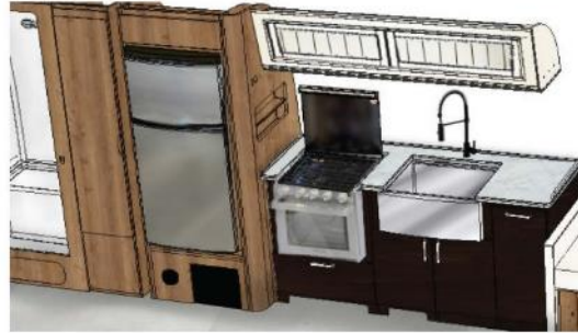
APPLIANCES Conv Micro: 690734 Description: Convection Microwave, 1.1 CUF MNF: Furion/Contour *NOT PICTURED LARGER* Norcold Refer: 690771-01 Description: 8.2 CUF, LH Hinge
