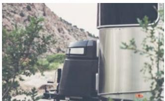
In order to keep the inside of the Basecamp safe, LP gas has to be stored in specific locations where it can't vent into the trailer. That's why we designed our own patented LP storage compartment and cover on the front of the Basecamp. It's made of a special thermal plastic that surrounds the entire LP system, and it's hollow, so if there is a gas leak, it will vent out the bottom and into the fresh air.
