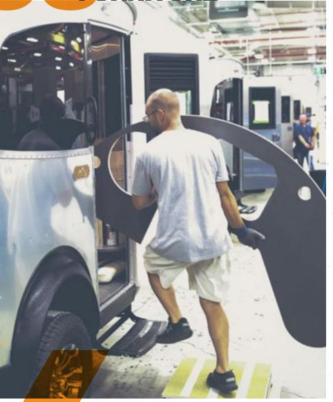
Once Basecamp's floor and walls are attached, everything has to fit through the front door or the rear hatch so as not to interrupt the integrity of the superstructure. That's why all of our furniture and cabinetry is handcrafted to fit the curves of the Basecamp perfectly. It's all residential quality, with solid wood assemblies instead of particle board and paneling.
