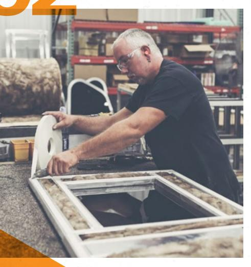
Once the outer structure is assembled, we install EcoBatt® insulation between the aluminum ribs, just like we do in our standard travel trailers. Not only does EcoBatt meet the tightest indoor air quality certification and performance standards in the industry, it's also made primarily from sand and recycled glass.
