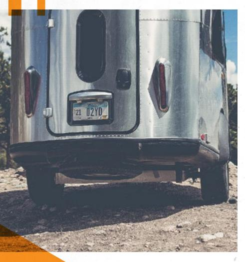
A departure angle is the degree at which your trailer meets the ground when you're coming down a hill. The steeper the departure angle on the trailer, the less chance the trailer has of scraping the ground. Looking at the Basecamp, you'll notice the departure angle right away. The back end slopes upward and includes skids underneath that keep the undercarriage from being damaged.
